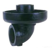
The use of an Apollo International<sup>™</sup> drip pan elbow is highly recommended for steam safety valve installations. The drip pan elbow connects to the valve outlet to safely direct steam discharge away from the valve and into the discharge piping. Condensate is directed to drain. Drip pans offer ideal flow characteristics, and serve to isolate the valve from piping stresses that can adversely effect safety valve performance and longevity.
